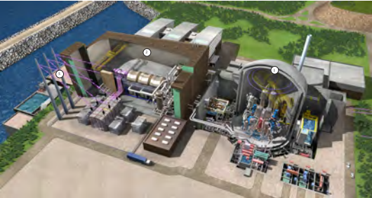
Illustrative UK EPR™ Nuclear Reactor and Turbine Hall layout SIZEWELL C - DESIGN REVIEW PANEL
